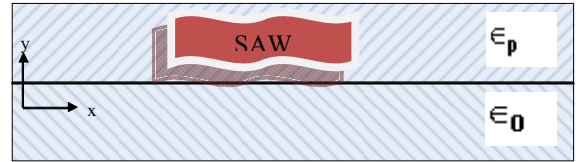
Figure 1 SAW propagation schematic for analysis.
